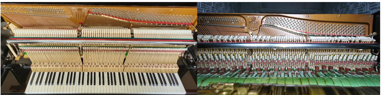
Foto – Photo: 5.5 Zoll / inch = 139,7 mm Untertasten / white keys ./ ca. 3,63 mm / Obertasten / sharps ./ ca. 2 mm
